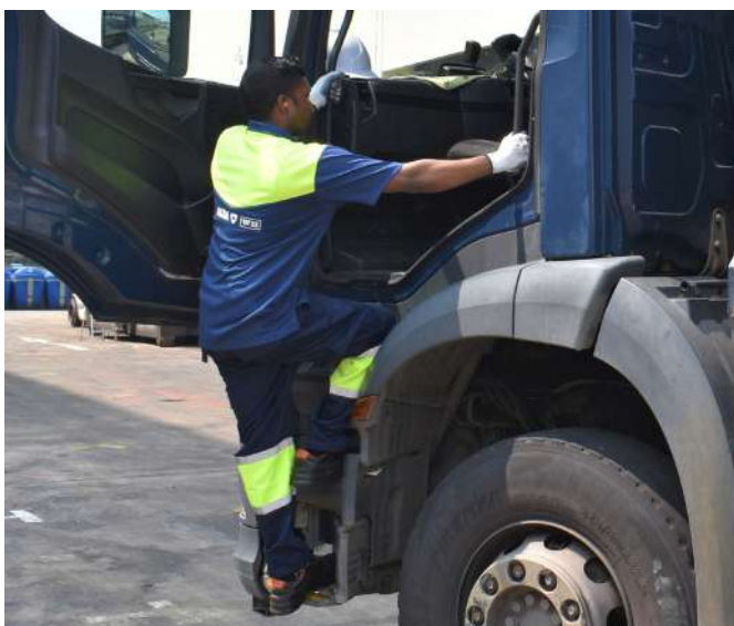
Figure 8: Handholds allow for three-point contact when boarding and disembarking
