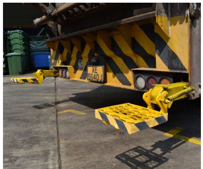
Figure 9: Proper footholds to access the rear of the waste collection vehicle
