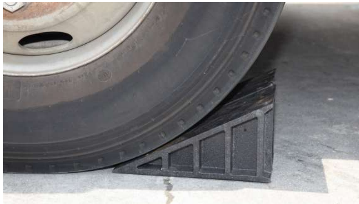
Figure 11: Wheels of stationary vehicles should be chocked
